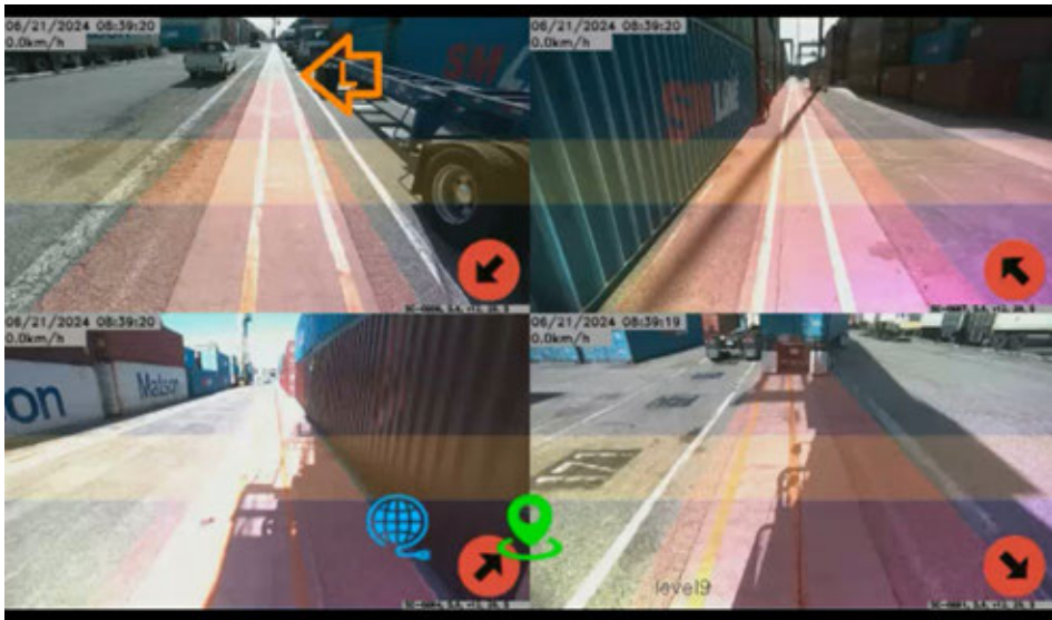
Strata’s HazardAI proximity detection system identifying vehicle, container, and pedestrian hazard zones in real time to support collision avoidance operations
